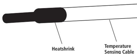
If temperature compensated charging is required, attach the ring terminal of the Temperature Sensing cable to the auxiliary battery terminal. For best results, attach the ring terminal to the auxiliary battery plastic surface with thermal conductive adhesive such as 3M TC-2810 or equivalent.
